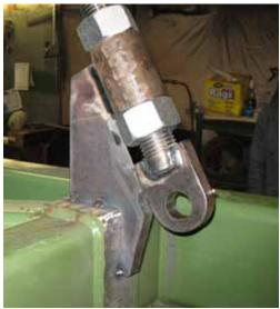
7) Next, re-install the cylinder onto the new lollipop. The rod end of the cylinder will be used to help place the bottom cylinder lug on the running gear leg.
