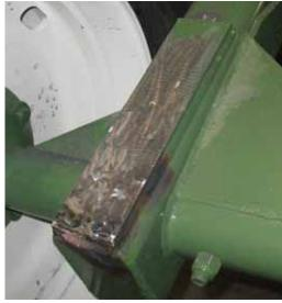
4) Take the lollipop alignment jig and clamp it in place on top of the wing frame as shown. The jig should straddle the upper base plate while resting on the top surface of the frame. Push the jig into the corner of the frame as far as it will allow and then clamp it. The jig will work for both the right and left wings.
