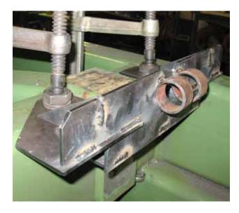
5) Pre-assemble the new lollipop to the new lollipop tower as shown, with a 2" nut on either side of the collar and with the lollipop resting on the flat protrusion (grease-zirk facing away from the weldment). Hand tighten the lollipop after adjusting the hole center to 5-5/8" from the front edge of the round tubing collar as indicated. Make sure the sides of the lollipop are flush with the sides of the tower (the lollipop should not be kinked to one side)
